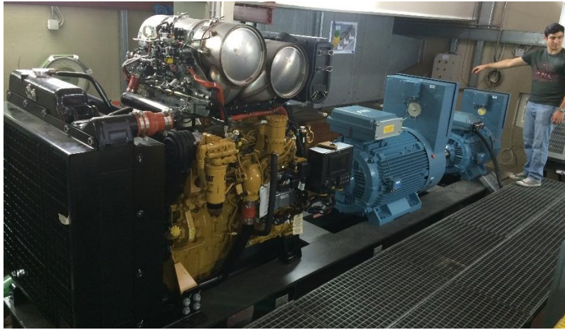
Fig. 7. All units as placed on the common bedplate.
