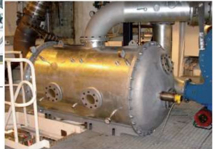
Fig. 16: The newly developed EGR scrubber applied to the test engine
